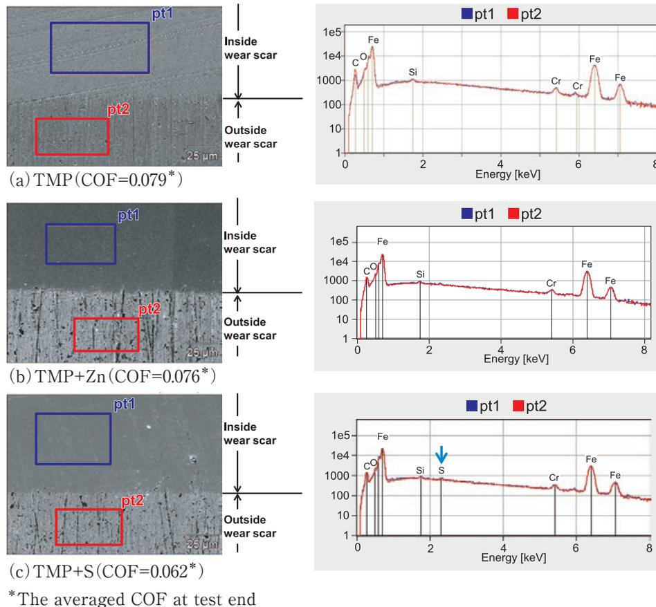
Fig. 9 SEM image and EDX spectrum on SUJ2 roller lubricated with TMP blended oils
