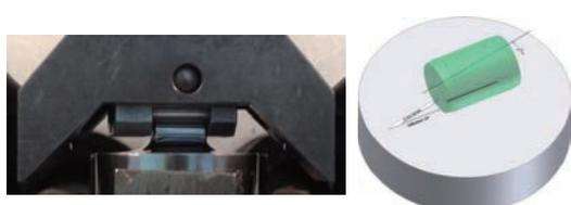
**Fig. 2** Standard inclined roller in SRV<sup>®</sup> tribometer
